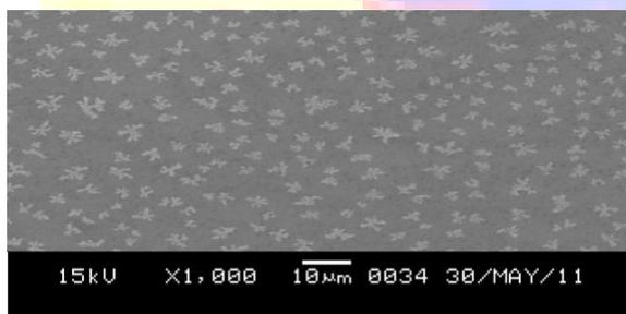
Fig. 3(c) : SEM micrograph of ZnS doped with Fe
