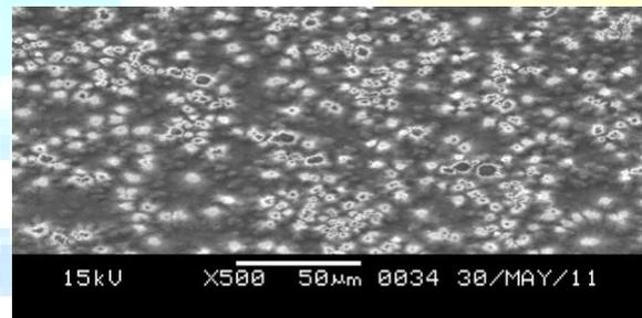
Fig. 3(b) : SEM micrograph of ZnS doped with Mn
